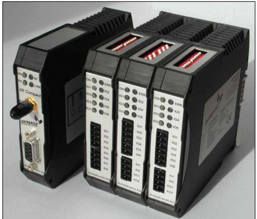
The modules are connected together by T-bus plugs.
